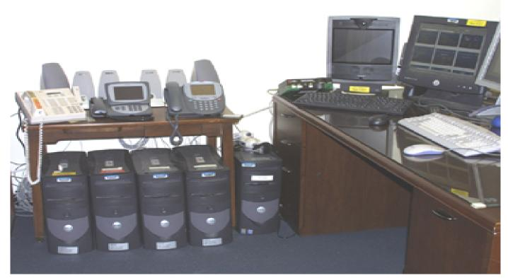
To ensure a high level of security physically isolated clients were deployed often resulting in up to 10 different PCs in a single office.
