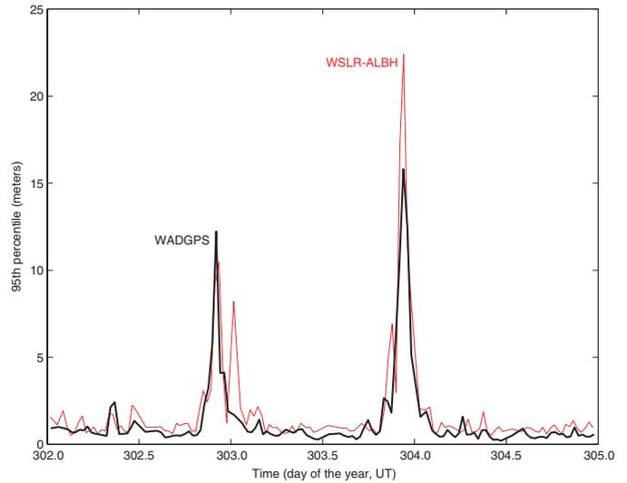
**▲ FIGURE 11** 95th-percentile DGPS horizontal positioning accuracies for the WSLR-ALBH baseline (red line) versus WADGPS results (black line) in Network 1, for simulated user WSLR.
