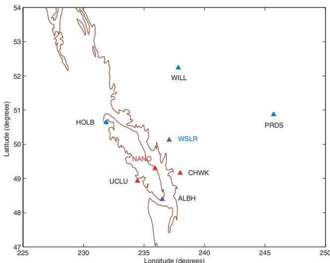
**Figure 2** Reference stations used for differential processing in western Canada. Simulated users are WSLR in Network 1 (blue triangles) and NANO in Network 2 (red triangles).
