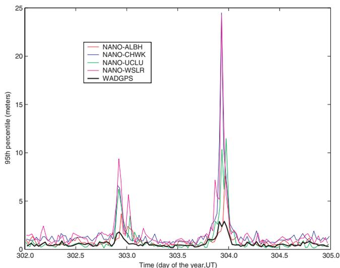
**▲ FIGURE 12** 95th-percentile DGPS horizontal positioning accuracies for baselines in Network 2 versus WADGPS results, for simulated user NANO.
