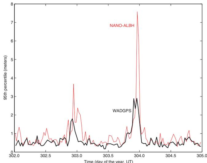
**▲ FIGURE 13** 95th-percentile DGPS horizontal positioning accuracies for the NANO-ALBH baseline (red line) versus WADGPS results (black line) in Network 2, for simulated user NANO.
