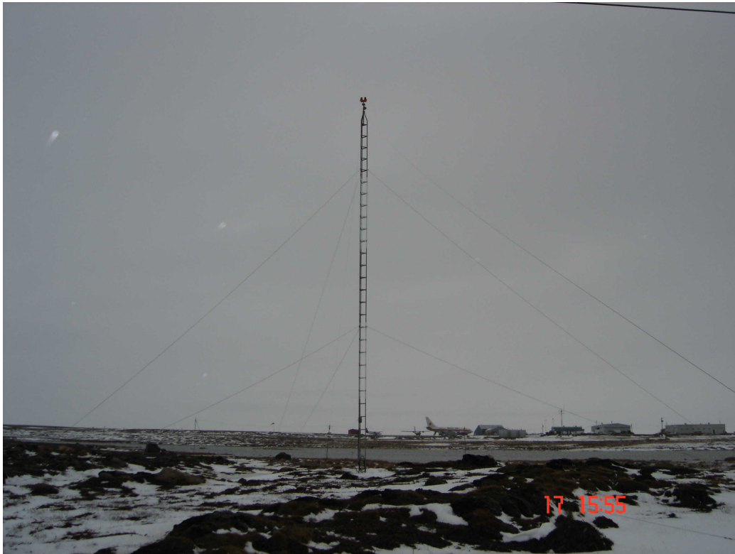
Figure 2.12: Canadian Advanced Digital ionosonde (CADI) installed in Cambridge Bay, Canada.
