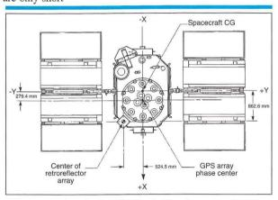
**Figure 3.** A sketch of a GPS satellite shows the locations of the retroreflector array, antenna array phase center, and the satellite center of gravity (CG). The positive Z-direction points out of the page.
