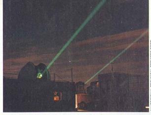
NASA MOBLAS-7 and a transportable SLR system were collocated at the Goddard Space Flight Center. A collocation is the most effective method of testing an SLR system for systematic errors.
