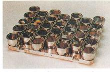
The laser retroreflector array used on GPS-35 and GPS-36 is made up of 32 individual retroreflectors that reflect light back in exactly the same direction from which it comes.
