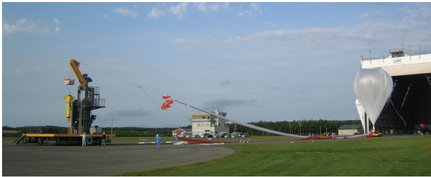
▲ FIGURE 1 Takeoff of the Balloon-based Operation Vehicle (BOV) 2009 experiment. The BOV and the gondola hanging from the sliding launcher can be seen to the left, while the balloon can be seen in front of the hanger on the right.
