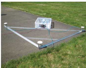
▲ FIGURE 6 Static experiment. Setup of the GPS antennas on the left; C-LAMBDA-based attitude estimates on the right.
