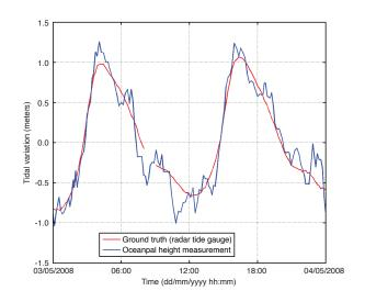
▲ FIGURE 6. Daily tidal variation at Scheveningen Pier, The Hague, The Netherlands, on May 3-4, 2008, measured by X-band radar and Oceanpal.
