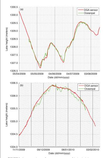
▲ FIGURE 5. A comparison of measurements of Lake Laja's water level by Oceanpal and a water bubbler sensor operated by Dirección General de Aguas (DGA) for two periods of time corresponding to (a) the austral winter (from late April 2009 until early August 2009) and (b) the austral summer (from late November 2009 until late January 2010).
