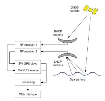
▲ FIGURE 1 Basic operation of Oceanpal and the principle of GNSS-R-based sea-surface monitoring. Right-hand and left-hand circularly polarized antennas feed signals to radio frequency (RF) receiver front-ends that, in turn, feed software (SW) receiver back-ends and subsequent processing algorithms.
