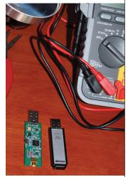
▲ **FIGURE 7** The USB sticktype front end for the iPRx receiver beside a standard USB memory stick.
