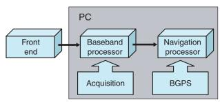
▲ **FIGURE 1** A block diagram of a PC-based snapshot software receiver, which has been developed to facilitate BGPS technology development and serves as a prototype for an airborne receiver. There are extra tracking loops for the airborne receiver, which are not shown here.
