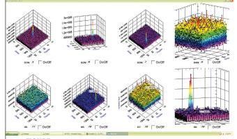
▲ **FIGURE 4** A screenshot of the iPRx software window showing acquisition selections. The horizontal axes represent code delay and Doppler shift. The plots are scalable and can be rotated to allow better visualization.
