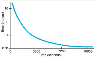
▲ **FIGURE 6** The approximate relationship between achievable accuracy of standalone positioning and the time required to achieve such accuracy. The regions where the plot converges to the axes represent the biggest challenges.
