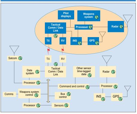
**Figure 2** Virtually all electronic systems onboard ships and aircraft contain oscillators and clocks. Some of these systems need only relative time but intercommunication between systems requires time coordination.
