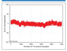
**Figure 4** The GPS Precise Positioning Service can provide time transfer precisions (one standard deviation) better than 10 nanoseconds.
