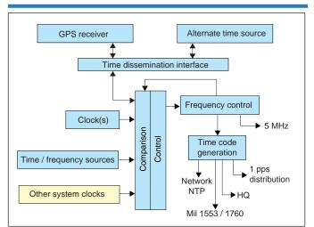
**Figure 7** The common time reference (CTR) functional infrastructure would include the necessary components for generation, comparison, maintenance, and distribution of the CTR within and across systems.
