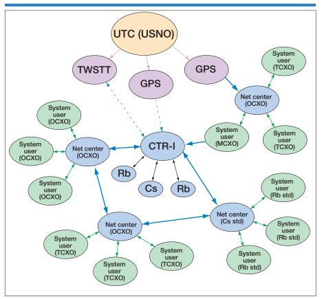
**Figure 6** The common time reference (CTR) architecture would incorporate existing clocks into a combined clock group. Groups would be compared with an independent local CTR (CTR-I) which, in turn, would be compared with the absolute CTR through GPS and other means.
