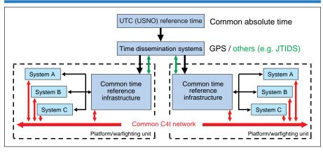
**Figure 5** In the common time reference approach, time is disseminated from a central source through GPS and other means to platform warfighting units connected to a common command, control, communications, computers, and intelligence (C4I) network.
