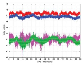
▲ **FIGURE 1** Carrier-power-to-noise-density ratio (C/N<sub>0</sub>). The magenta and green dots represent the PRN135 C/N<sub>0</sub> values for L1 and L5, respectively. The red and blue dots represent the PRN 138 C/N<sub>0</sub> values for L1 and L5, respectively.
