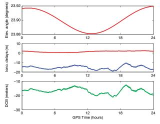
▲ FIGURE 6 Computed satellite and receiver combined DCB for WAAS PRN 138 on August 25, 2008. In the second panel, the red dots show the computed ionospheric delays using WAAS ionospheric corrections and the blue dots represent the carrier-phase-leveled ionospheric delays.
