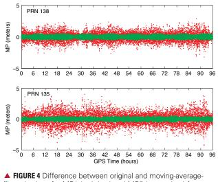
filtered values for MP1 (red dots) and MP5 (green dots) for PRN135 and PRN138 for August 24–27, 2008
