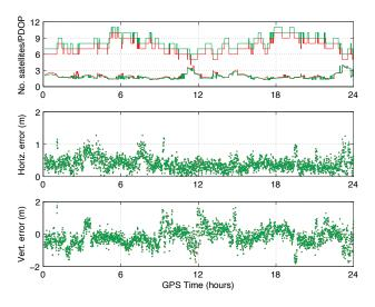
▲ **FIGURE 8** Benefit of using WAAS GEO ranging in point positioning. The top panel shows the number of satellites that have been used for the point positioning process and PDOP and the lower panels show the positioning results. The green traces and points show the results of using GEO ranging data and the red traces and points show the results without using WAAS GEO ranging measurements.
