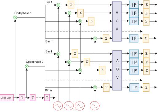
**Figure 2** A two-code-phase subATTO search engine. In addition to the operational blocks described in Figure 1, the ACV (autoconvolution) block constitutes a proprietary algorithm utilizing multiple fast Fourier transform (FFT) bins. The FFT/ACV/squarer process provides improved sensitivity for the same overall integration period compared to the technique of Figure 1.
