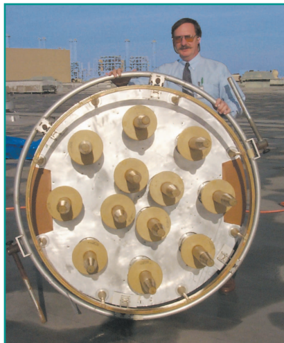
FIGURE 1 The first author holds the Block IIA antenna used for these tests, showing the location of the transmitting elements.
