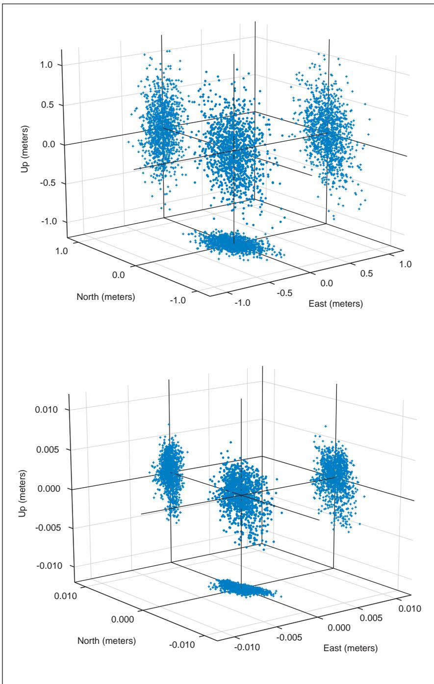
**Figure 1.** Relative positioning results on a short baseline are expressed in east, north, and up components. Shown are 1,200 single-epoch solutions for the case with ambiguities real-valued (top) and fixed (bottom). For the fixed solution, the ambiguities are resolved correctly in all cases. Fixing the integer ambiguities incorrectly would generally shift the position solution by a decimeter or more. After successful fixing, the precision of the coordinates is below the 1-centimeter level.
