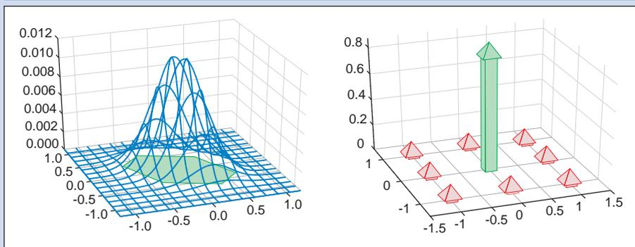
By taking the integral of the probability density function (on the left) over the pull-in region for each integer vector, the probability that this vector will result as the integer least-squares solution is obtained. The probabilities are given on the right for the integer vectors between -1 and +1. The integral over the area for the correct integer vector, in this case (0,0), gives the success rate. It is about 85 percent in this example.
