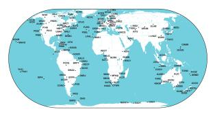
▲ **FIGURE 1** GNSS tracking stations in the IGS real-time network.
