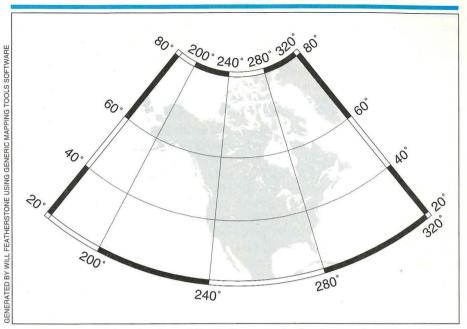
**Figure 3.** The Lambert Conformal Conical map projection is one of many projections devised in the eighteenth century by J.H. Lambert. All meridians are represented by equally spaced straight lines, and the parallels of latitude are represented by a series of unequally spaced arcs of concentric circles. This projection has been used extensively for mapping regions with a predominantly east–west expanse.
