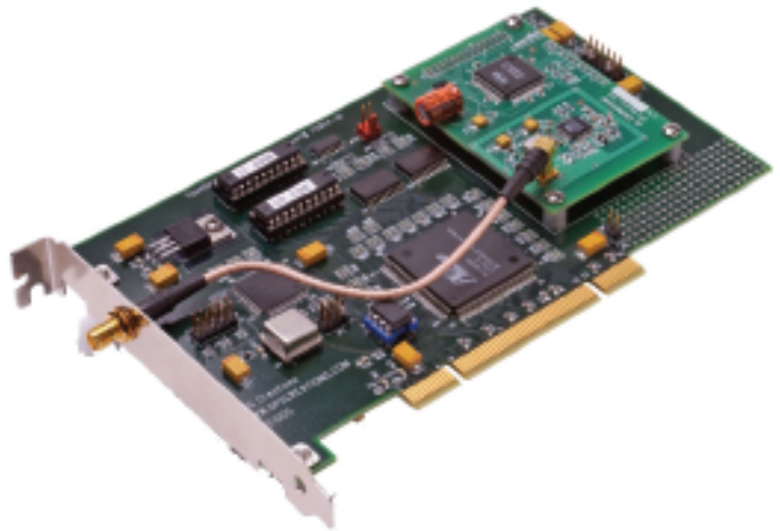
▲ PHOTO 4 GPS 1005 PCI interface with daughter board
