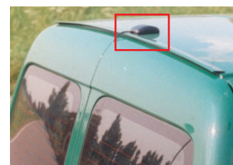
The external antenna mounted on the back of the van. The roof is about 1.8 meters above the road surface.
