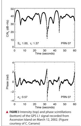
observed carrier phase obtained from the receiver's phase lock loop. These same irregularities can cause increased phase noise, cycle slips, and even loss of lock if the phase fluctuations are too rapid for the receiver to track.
