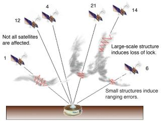
▲ FIGURE 4 Schematic of the varying effects of scintillation on GPS.
