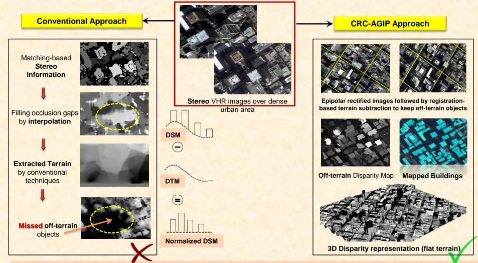
**Description**: The algorithm forces the matching techniques to map only the disparities of building rooftops by subtracting the terrain level features in the image space. It also takes the advantages of along-track stereo images of opposite directions to exclude building facades. The product of this algorithm is a disparity map that contains only the building rooftops. The algorithm is well suited for dense urban areas since the terrain variation is reasonable.
