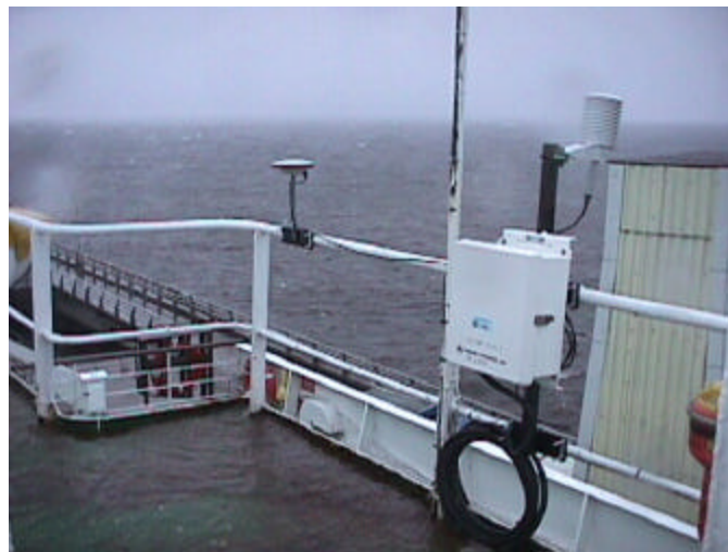
Figure 12 – GPS receiver and meteorological station on board
