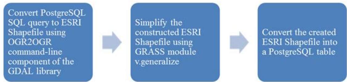
Figure 0.3: Flow diagram to construct a simplified trajectory using Douglas–Peucker algorithm
