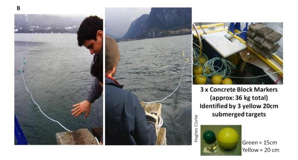
Figure 3.4 – Showing the block markers and targets (A) and their deployment (B)
