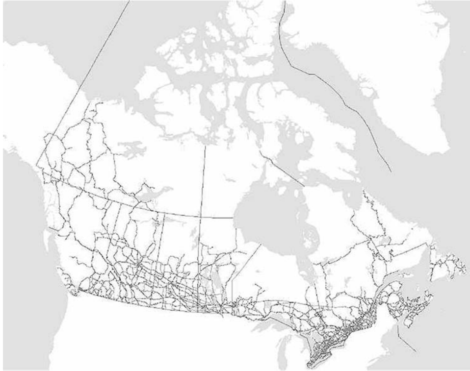
FIGURE 6 The Canadian national geodetic levelling network (Source: www.nrcan.gc.ca . Copyright: Her Majesty the Queen in Right of Canada, Natural Resources Canada, Geodetic Survey Division. All rights reserved.)
