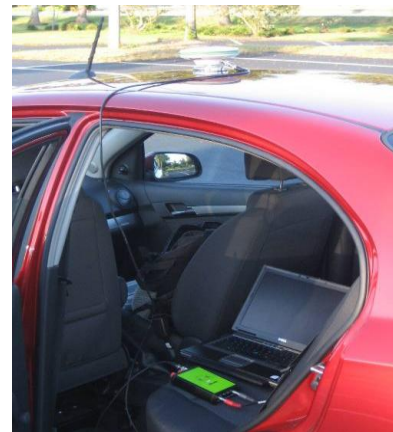
Figure 2: Kinematic test setup
