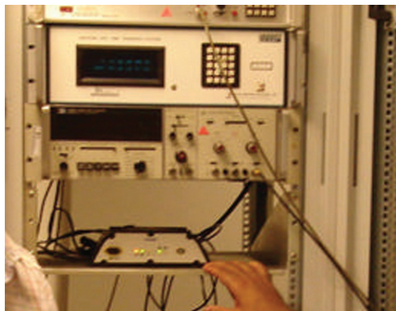
Fig. 3 New receiver of the ONRJ station with atomic clock
