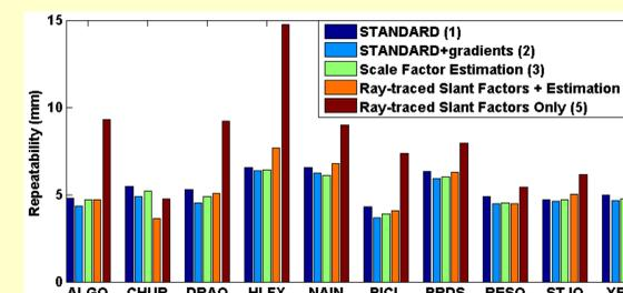
Figure 4.0 Repeatability of station solutions in up direction for Jan. 1-14, 2008
