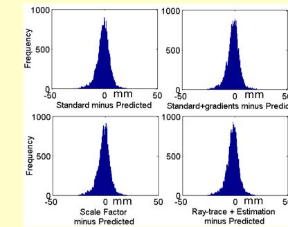
Figure 6.0 Distribution of estimated residual delays after convergence has been achieved (3 hours) w.r.t. predicted delays. Units of mm.
