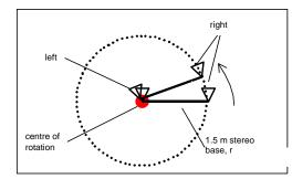
Figure 3. Overhead view of rotating panoramic and stereo-pair image acquisition
