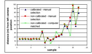
Figure 4. Comparison of manually-derived (calibrated, non- calibrated) and computer-derived distances (stereo pair 1, test location B)
