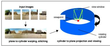
Figure 1. Overview of cylindrical panoramic imaging process
