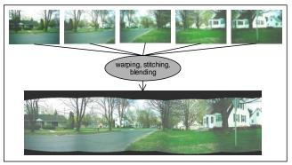
Figure 4. Sample results of automatic warping, stitching, and blending for cylindrical panorama creation for test site B
