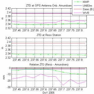
Figure 12 – ZTD at moving antenna (upper plot); ZTD at Reso station (middle plot); relative ZTD (lower plot)
