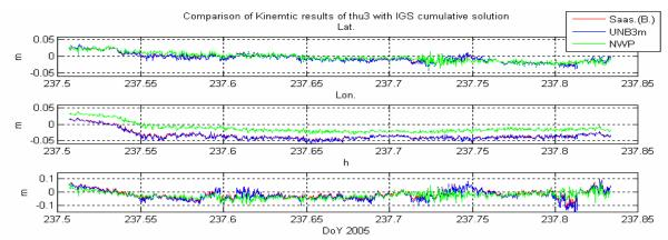
Figure 11 – Comparison of thu3 kinematic result of three neutral atmosphere strategies with IGS cumulative solution
