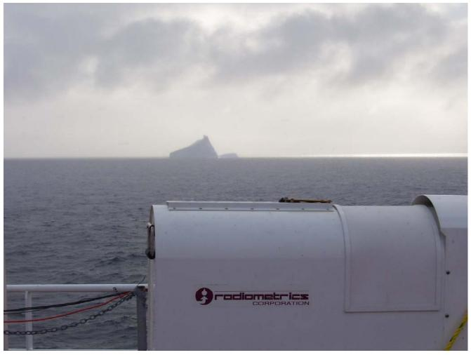
•The water-vapour radiometer delivers an atmospheric path-length correction based on integrated water vapour.
