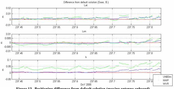
Figure 13 – Positioning difference from default solution (moving antenna onboard)
