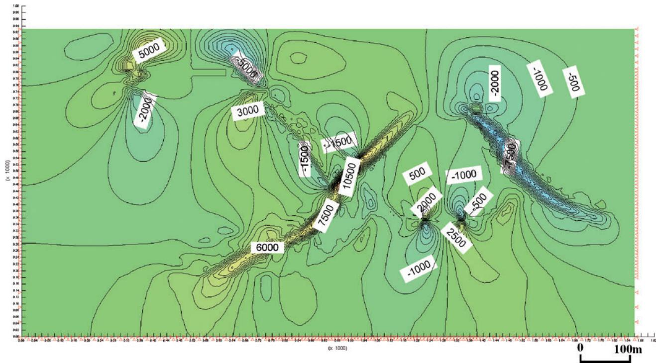
Figure 7: Distribution of maximum shearing stress [MPa].
