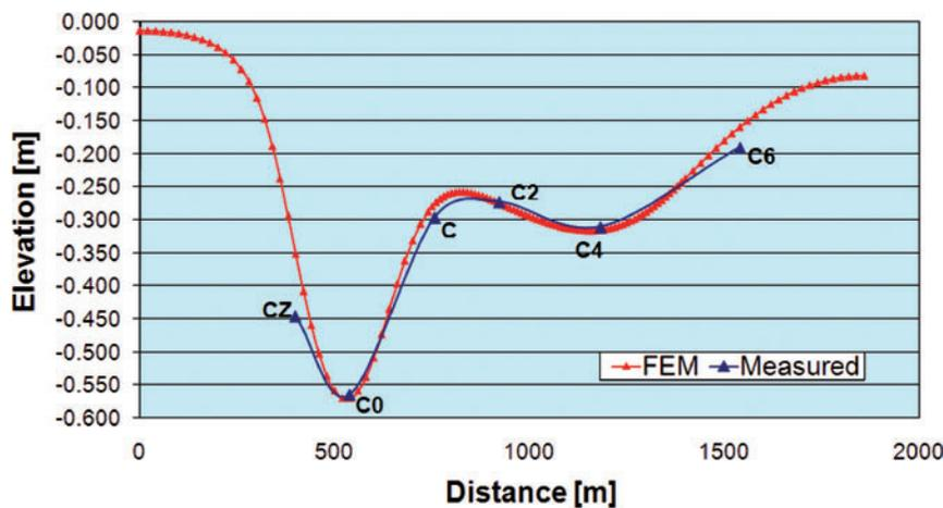
Figure 6: Measured and FEM surface subsidence.
