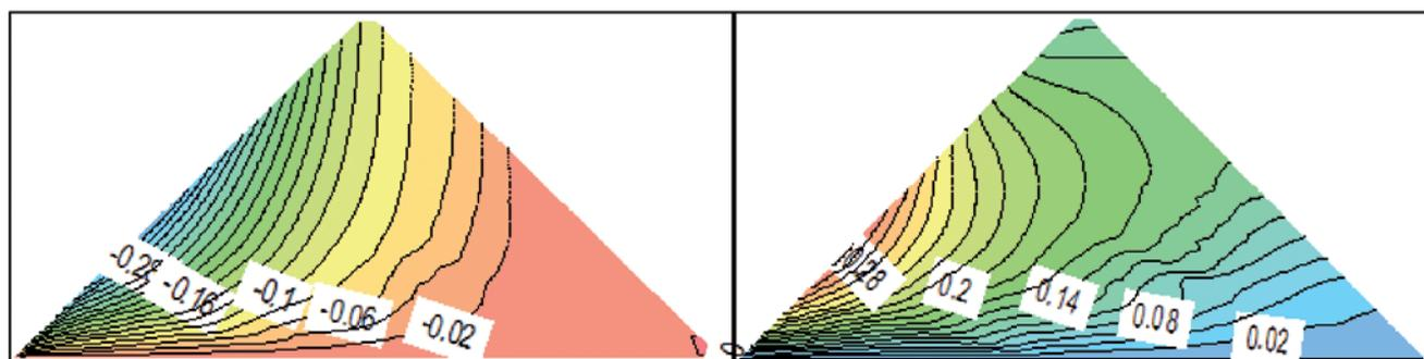
Figure 2: Predicted displacements [m] after filling the reservoir. a) vertical displacements, b) horizontal displacements.
