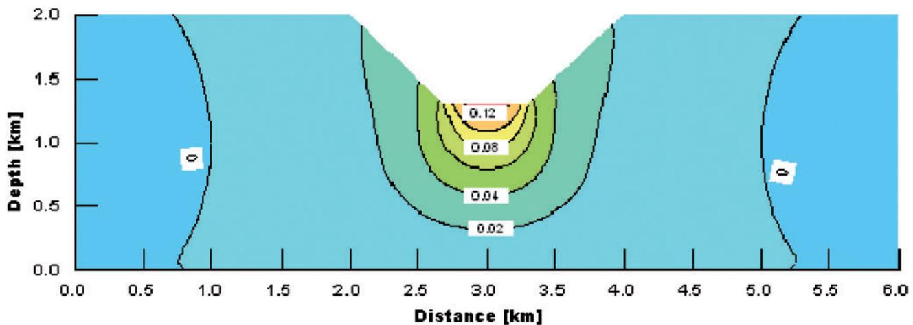
Figure 3: Vertical displacement [m].
