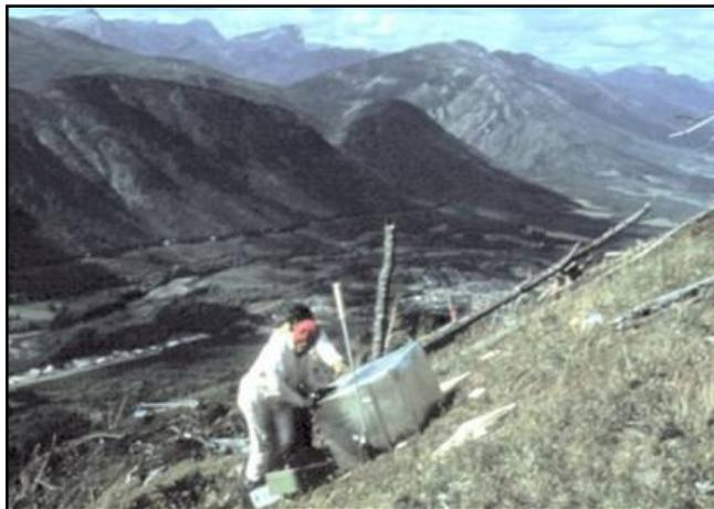
Fig. 2: Installing tiltmeter station
