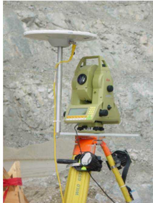
Figure 6 A stand alone RTS with GPS on the pit floor
