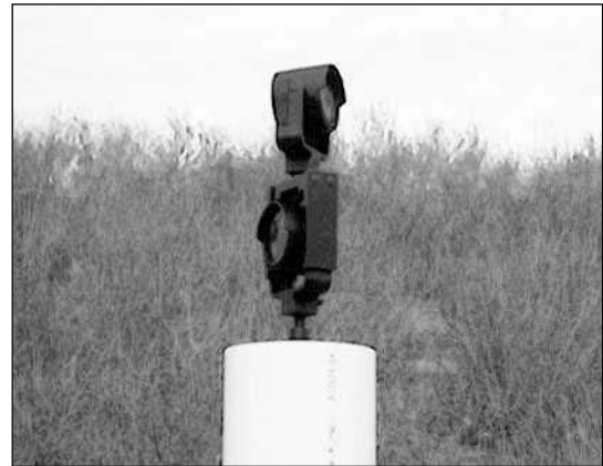
Figure 3. A dual SMP installation at a control point.
